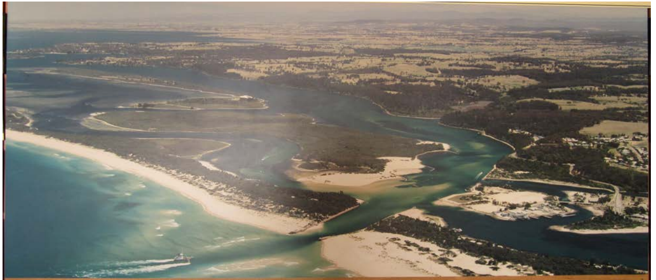
The Entrance before August 2008 deepening. It shows the numerous sand bars which slowed the ingress of salt water.
